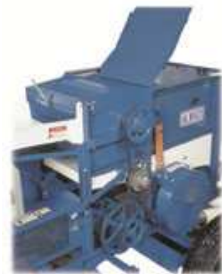
Fully enclosed, variable speed threshing cylinder is standard equipment.
