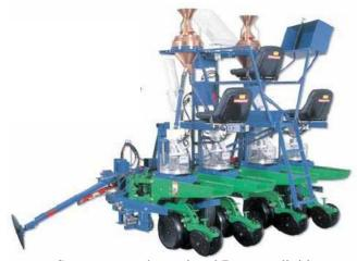
Set up to use the optional Boerner divider system, electric seed try indexer, or to plant individual rows. Equipped with cone type seeders, roller checkhead system or cable winder, and single telescoping toolbar. Shown with John Deere row units, Kinze Row units also available.
